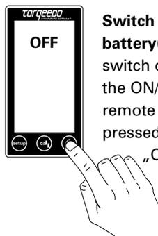
**Switch off the motor and battery(ies):** In order to also switch off the battery, keep the ON/OFF button on the remote throttle or tiller display pressed for 5 seconds until "Off" icon is displayed.
