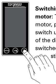
**Switching off only the motor:** To switch off the motor, press ON/OFF switch until blackscreen of the display: motor is switched off, batteries still run.
