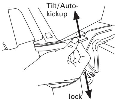
The tilt lever in the “tilt/auto kick-up” position (lever up) enables the motor to be kicked up if it touches the bottom. In this position it is not possible to reverse at full speed or to stop the boat.
