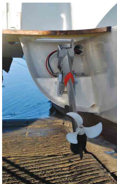
Xhale off Frazer Island. (top) Lithium batteries in situ. (above left) Torqeedo motor controls. (above right) Torqeedo electric motor – transom mounted. (above)
