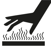
Caution: hot surface
