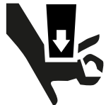
Caution: crushing hazard
