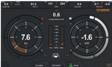
Drive screen: All important information needed while motoring or sailing. You can choose to display or hide the information line at the top.
