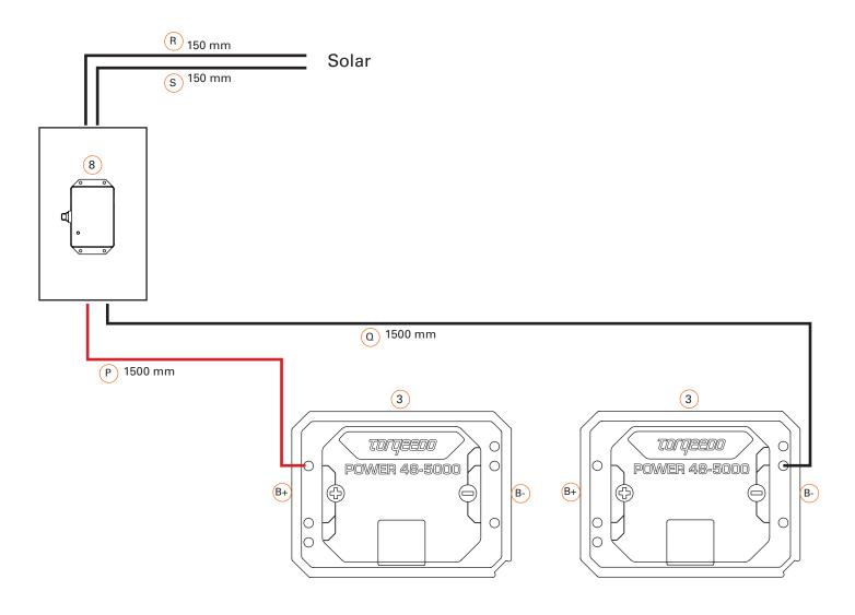
Positive power cable Negative power cable Positive charging cable Negative charging cable
