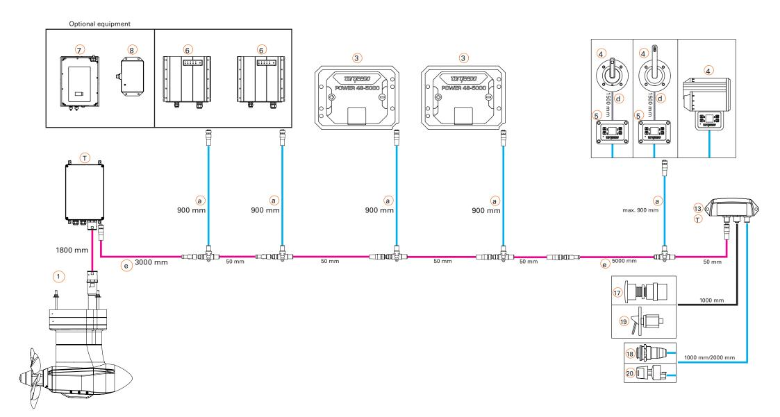
Backbone TorqLink, 8 pin data cable
