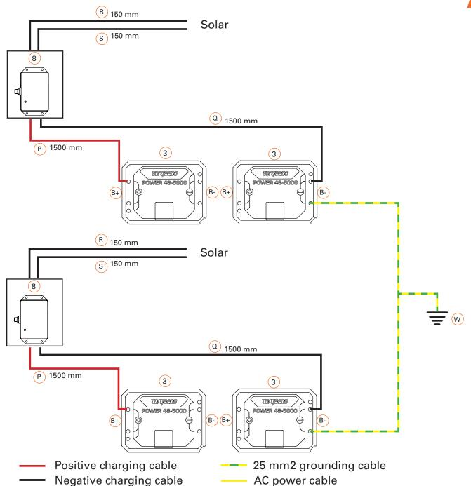
Positive power cable Negative power cable Power cable connection
