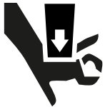
Caution: crushing hazard
