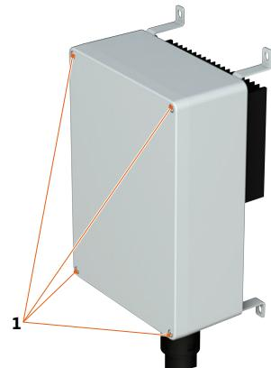
Fig. 44: Schroeven elektronicabox
