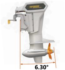
Fig. 56: Motor is tilted fully downwards
