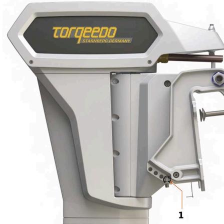
Fig. 43: Securing cotter pin for trim rod
