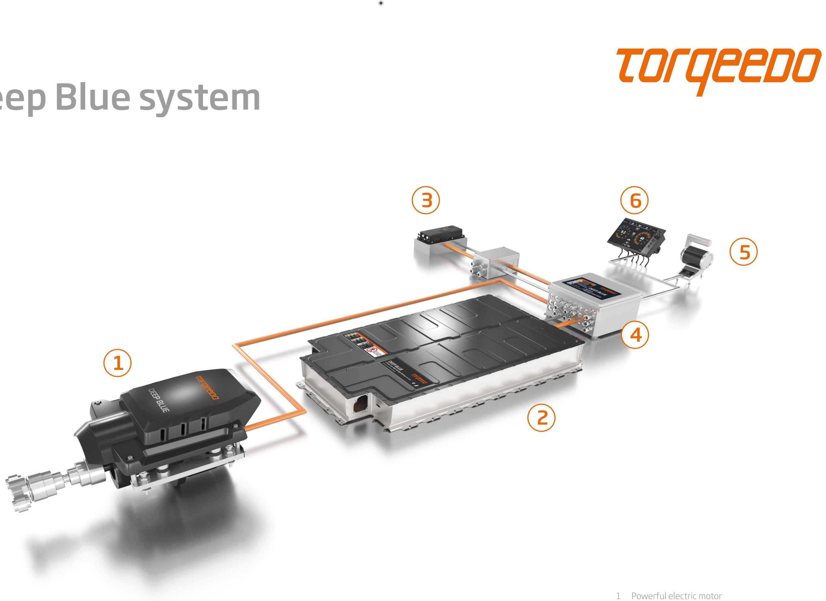
2 360 V high-capacity lithium battery system 3 Shore power chargers 4 System management unit5 Electronic throttle 6 Display with onboard computer
