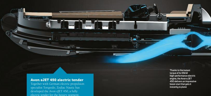
Equipped with Torquedo's 55kW Deep Blue electric motor and a modified version of the 30.5kWh lithium-ion battery used in BMW's i3 electric city car, the eJET gets around 90 minutes of range at 23kts (26mph) or seven hours at 5kts (5.7mph), and achieves a maximum speed of 31kts (35.6mph). The Avon eJET 450 also carries connected capabilities, meaning it can be maintained and upgraded directly through the internet.
