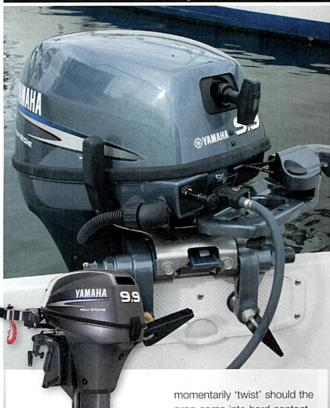
THE much copied Yamaha is neatly designed and has a good carrying handle. Ours had a smallish gear lever on the starboard side of the engine, but a version with it on the side of the tiller arm is also available, which would be better for auxiliary use on a sailing boat.
