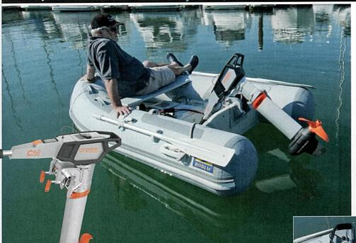
THIS is a brand new model from respected electric outboard builder, Torqeedo. As a comparison to the 10hp petrol outboards, the thrust from this unit is claimed to be comparable, which makes it a genuine alternative to a petrol outboard for a yacht's tender, RIB or small cruising craft up to four tons.
